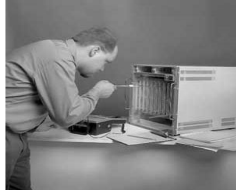
The above photo shows the traditional method of measuring airflow. It is tedious, inaccurate, and measures only one point at a time.
